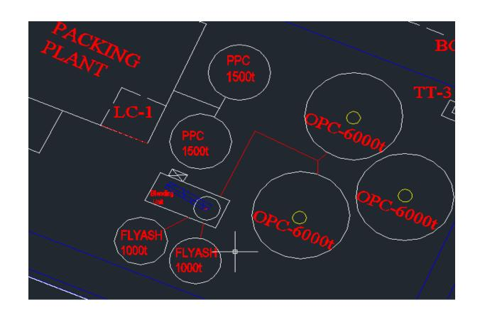
"Cement will be stored in 3 nos. silos of 6000t capacity each in RCC construction"
