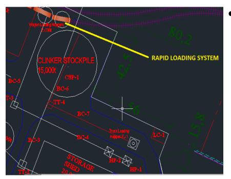
Clinker dispatch by wagons are proposed by rapid loading system (RLS) where 2 x 700 m³ steel hopers will be constructed above the proposed railway track (After extension of existing track) which will be able to load 40-42 wagons in one hrs time.
