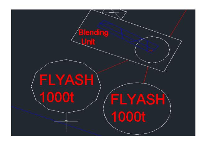
"Flyash silo shall be in steel construction capacity 2 X 1000 t with proper aeration & ventilation system"
